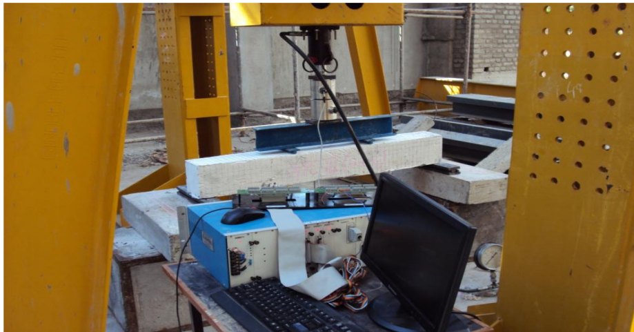
Fig 12 Experimental test setup of High strength GPC flexural member
