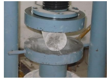
Fig 5 Testing of cylinders in CTM
