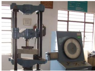
Fig 6 Rupture of prism in flexure test
