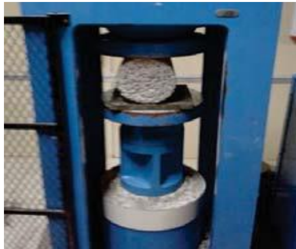
Fig 3. Split tensile strength test
