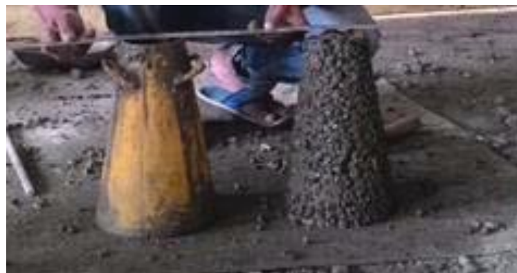
Fig 1. Slump cone test
